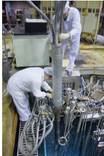
Fig. 6. An ampoule with SGFR fuel elements loading into the reactor
